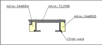
The advantage of the Cargo Floor SLP floor solution with exchangeable channel is that in case of extreme pollution of the channels these can be removed for cleaning without demounting and mounting the complete floor.
