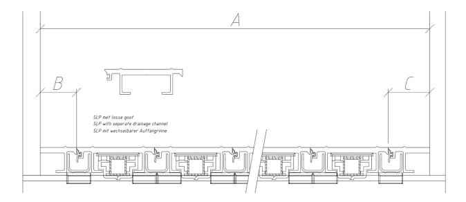
It is better not to weld the stationary edge profiles completely to the sidewalls, since at a later stage the floor may need to be retensioned, and to do this the side planks need to be loosened.
