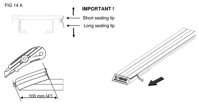
To aid the mounting of the seal, snip / cut about a little into the T-form at about 100 mm. [4"] from the start (this will form a handgrip, see figure 14 A).
