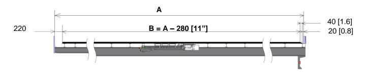
After cutting the floor profiles to length they need to be rounded-off (beveled) at the front as to ensure a smooth guiding of the floor profile while sliding in, and to prevent damage to the plastic bearing. To aid mounting, the rounded-off (beveled) side needs to lie in the mounting direction of the vehicle.
