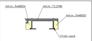
Next the side closing profiles (alu side closing profile L.=220mm SLP seal side, art. no. 5448004 and alu side closing profile L.=220mm SLP NOT seal side art. no. 5448005) can be placed in the profile and against the end block. Press the closing profile well against the profile and the end block. Now weld both closing profiles starting in the middle with three chain welds of about 40 mm. [1.6"].
