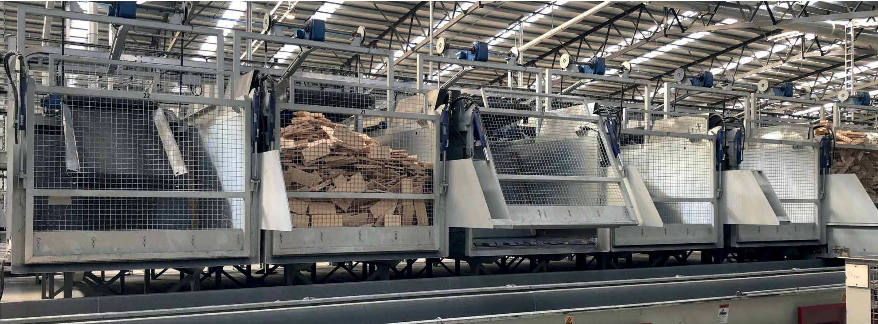
Step 1: all three hydraulic cylinders move the entire floor in the selected direction, thereby moving the product.
