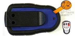
In order to have the hand transmitter communicate with the receiver you need to program the receiver. Open the lid of the receiver carefully. This is done by loosening the four screws of the receiver lid.
