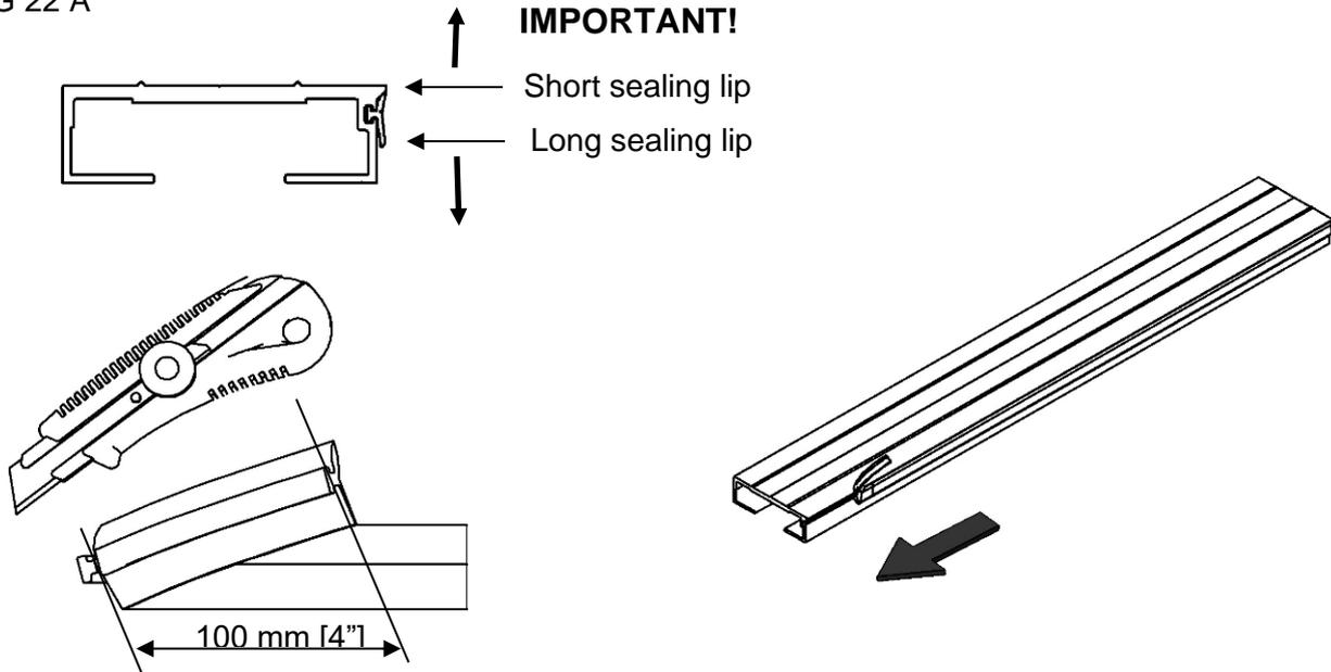
To aid the mounting of the seal, snip / cut about a little into the T-form at about 100 mm. [4"] from the start (this will form a handgrip, see figure 22 A).
