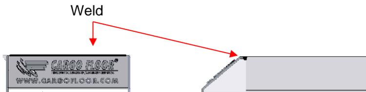
**SECURING THE FLOOR PROFILES TO THE DRIVE UNIT**
