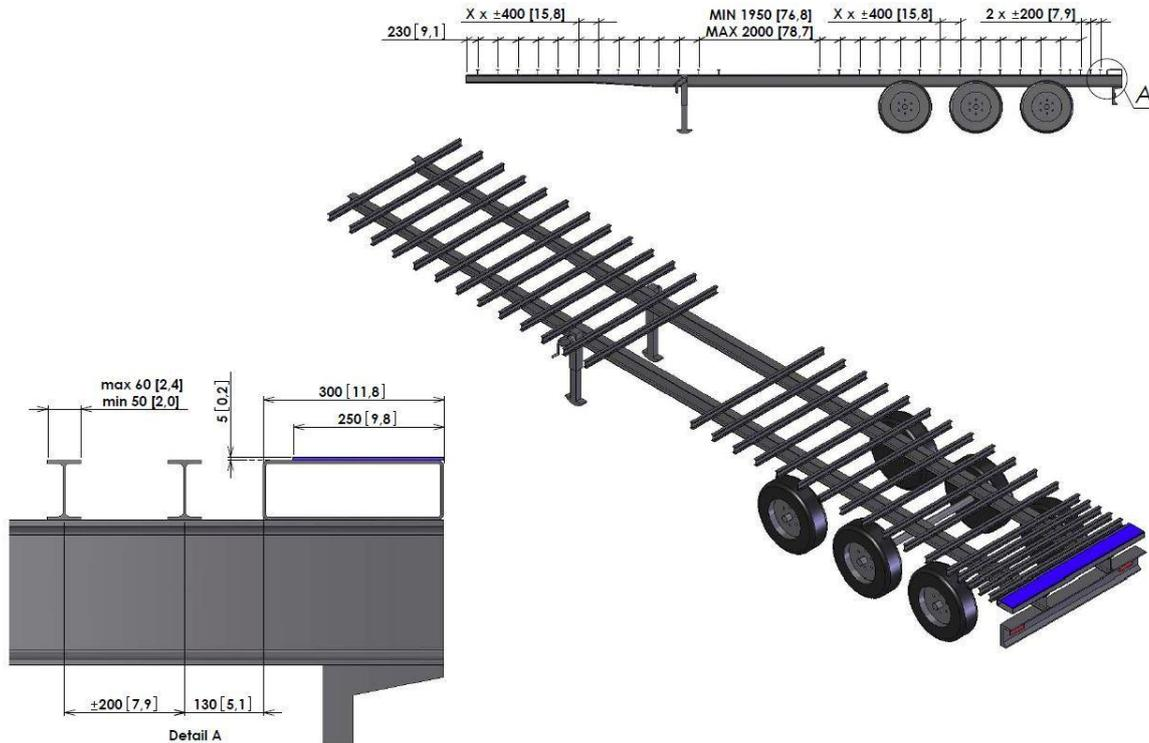
**When using the plastic bearing on the 25x25x2 [1"x1"x0.08"] square tube**
