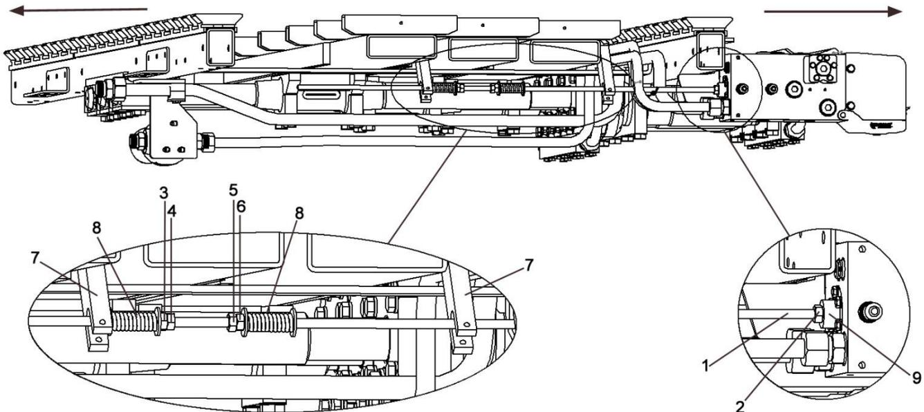
All Cargo Floor systems have the threaded rod set and are fully tested. You therefore do not need to adjust the threaded rod, but in certain circumstances (f.e. certain repairs) it may be necessary to check or adjust the setting of the threaded rod. If switching spontaneously doesn't go normally anymore, then please make a good assessment first why this has happened.
