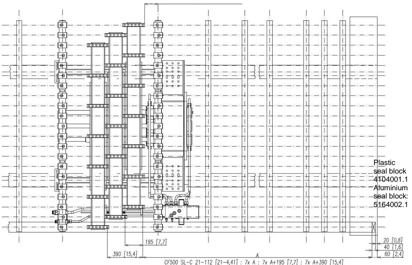
**DRILLING THE HOLES IN THE FLOOR PROFILES**
