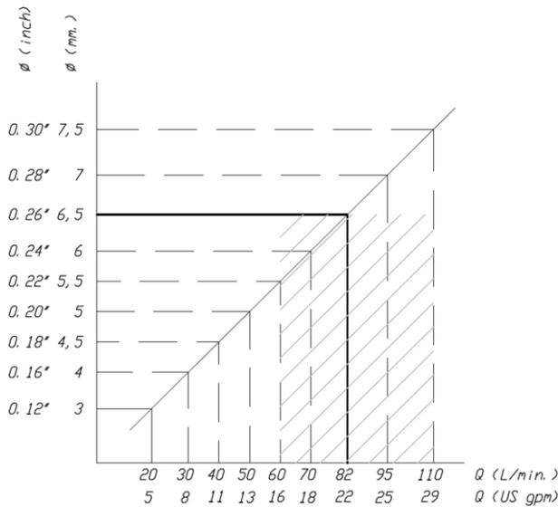
The shading points out the reach of the standard choke.
