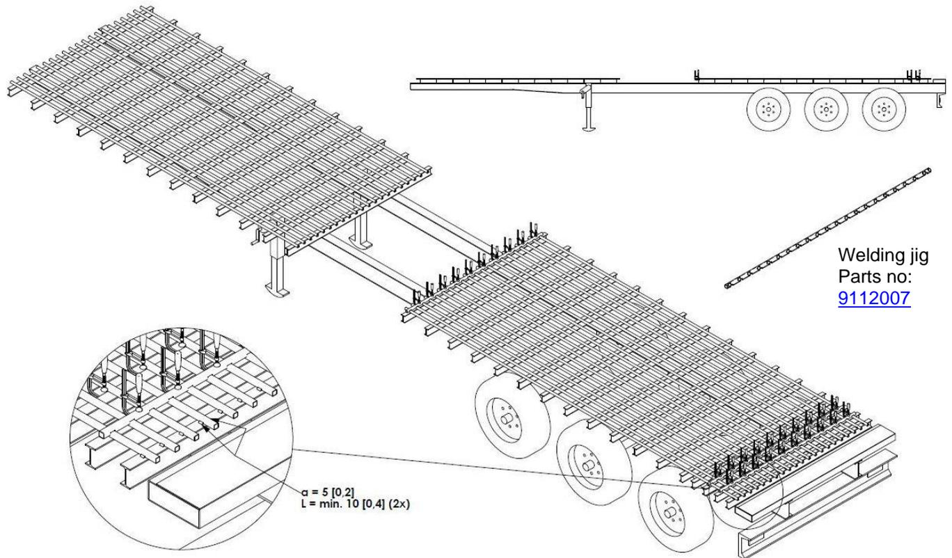
**MOUNTING THE U-PROFILES 25X25X2 [1"X1"X0.08"]**
