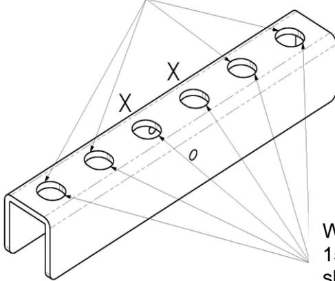
With special moving cross members (15/160 [6.3"], 15/156,8 [6.17], 18/112 [4.41], etc.) the profile should be fastened with 6 screws
