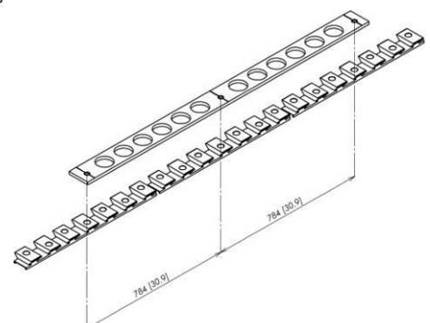
**CUTTING THE FLOOR PROFILES TO SIZE**
