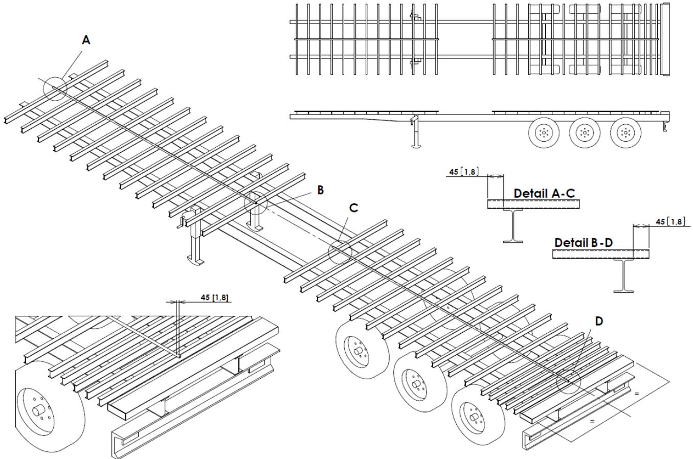
After this, all other tubes need to be mounted in exactly the same manner as the middle tube. Use the welding jigs (3 pieces, parts no. 9112007) for the right positioning of these tubes. All square should be - onside and in the same direction - pushed into the welding jig. The jig needs to be fastened securely to the crossmember to no height differences can occur between the square tubes. See fig. 4 B for positioning and use of the welding jigs.
