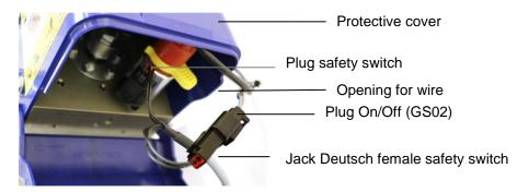
Pull the black plug out of the On/Off solenoid GS02 (the solenoid with the red emergency control). This can be done by pressing the locking clip of the plug and simultaneously pulling the plug. This plug needs to be plugged into the black jack, female, of the safety switch cable until the locking clip has clicked into the locking. Now plug the remaining black safety switch plug in the jack of the On/Off solenoid GS02.
