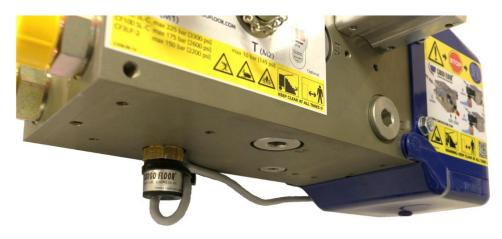
This concludes the installation of the Cargo Floor oil temperature safety switch.
