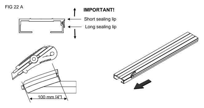
To aid the mounting of the seal, snip / cut about a little into the T-form at about 100 mm. [4"] from the start (this will form a handgrip, see figure 22 A).
