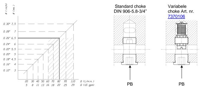
The shading points out the reach of the standard choke.
