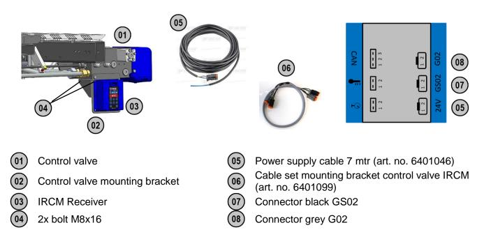
Mounting the IRCM Receiver to the control valve:
