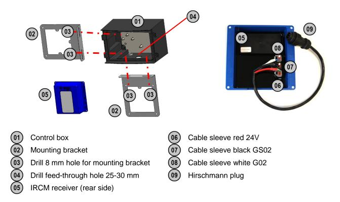
Mounting IRCM receiver mounting bracket to the Control box: sideways or at the bottom.
