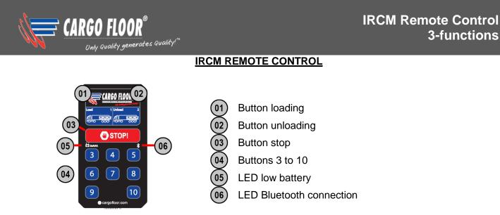
The remote control features Bluetooth technology and has two AAA batteries. The remote control is equipped with key illumination at the load/unload buttons if activated. When operating the buttons, a vibration will be felt. Do not put the remote control in your pocket to prevent unwanted operation and fast battery discharge.
