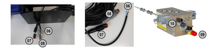
Pull the wiring for connection GS02 and G02 to the control valve. Connect cable GS02 (black plug) to the solenoid with the red cap [09]. Connect cable G02 (grey plug) to the solenoid with the black cap [10]. Pull the power supply cable [06] to the power supply. Connect the power supply as follows: Cable brown is +12-24V Cable blue is - 0V
