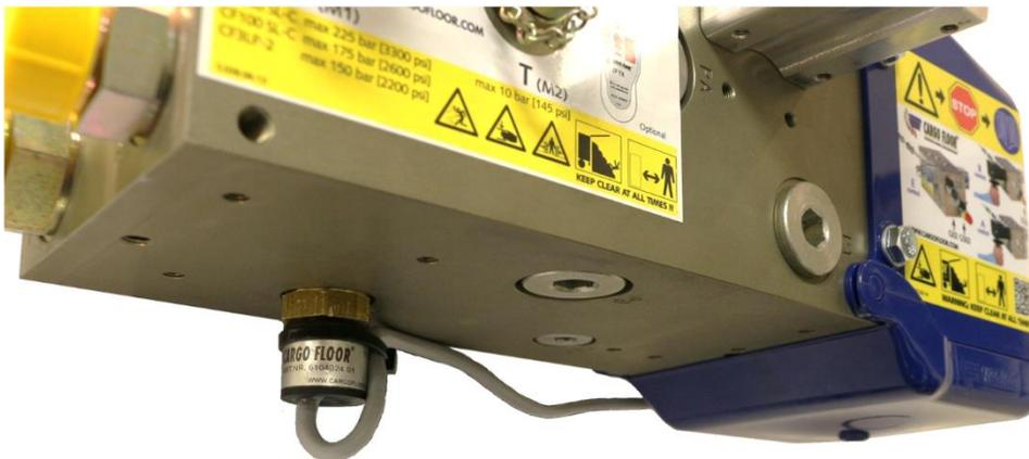
This concludes the installation of the Cargo Floor oil temperature safety switch.
