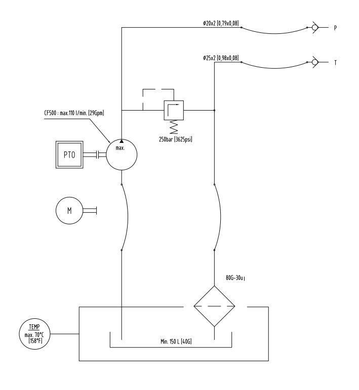
Aansluiting / Connection / Anschlüsse
