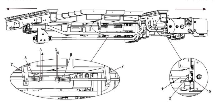
All Cargo Floor systems have the threaded rod set and are fully tested. You therefore do <u>not</u> need to adjust the threaded rod, but in certain circumstances (f.e. certain repairs) it may be necessary to check or adjust the setting of the threaded rod. If switching spontaneously doesn't go normally anymore, then please make a good assessment first why this has happened.
