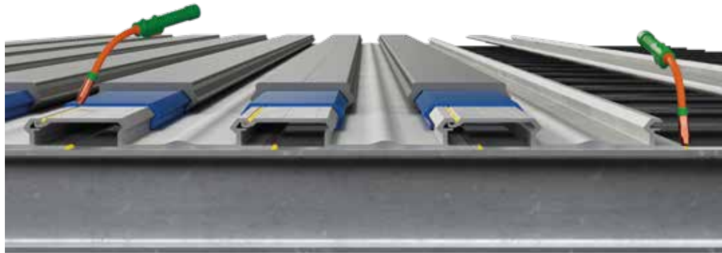
"Slide in" subdeck profiles welded on aluminum crossmembers (alternatively rivited), sealed by full length welds.
