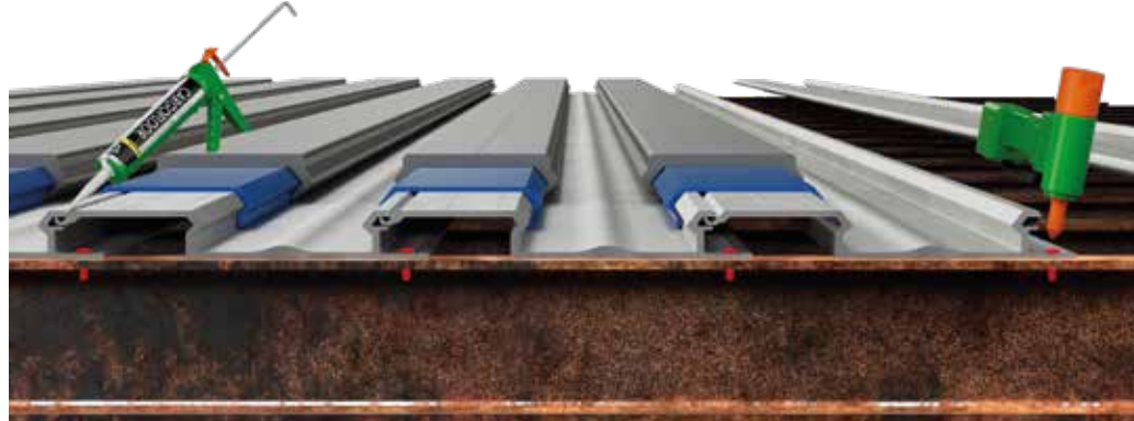
"Slide in" alu subdeck profiles rivited on steel crossmembers and sealed with sealant.
