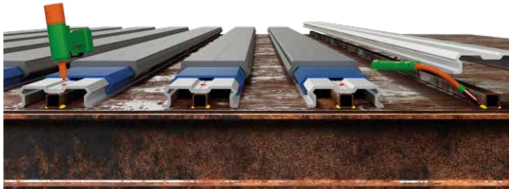
Loose aluminium subdeck profiles rivited on a steel box section welded to a steel plate.
